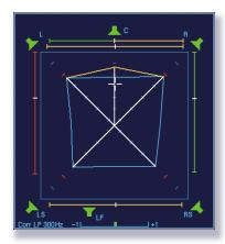
Surround signal with some Center presence, visible at the roof of the yellow line. A support microphone would be too dominant, a dialog in relation to music too quiet. The width of the PSI lines of the C channel is a sign of coherent signal parts in L and/or R (crosstalk).
