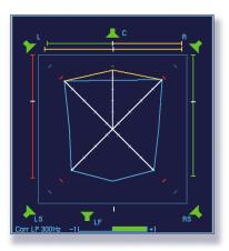
The widely outward broken TVI line between the channels LS and RS, no spread of the PSI line and the correlation level r=+1 in the lower phase meter indicate that an identical mono signal is applied in both surround channels. With these indicator elements also backward panned front channel parts can be detected.
