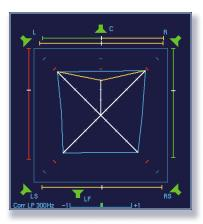
Surround signal with a low level of Center presence, visible at the downward broken yellow line. When recording music, the intermixture of a support microphone may enhance the perceptibility of the C channel in relation to the channels L and R. The correlation: for L - C is r > +0.25 (green), for C - R is r about 0 (yellow)
