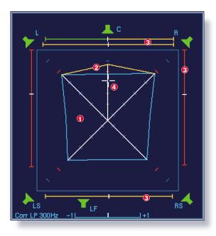
Direction and width of front, side, and rear phantom sources are represented by lines between the loudspeaker symbols – the Phantom Source Indicators (PSI). Their color changes with channel correlation.
