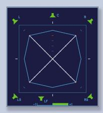
Identical sine wave signal with same level in the channels L, R, LS and RS, set to the referece monitoring sound pressure level. In each case the correlation is  $r=+1 \ (\text{hard outward broken TVI lines}),$  the phantom sound sources are exactly in the middle, similar to Mono signals.
