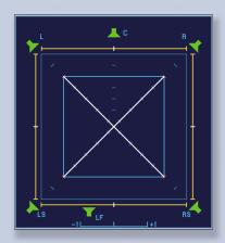
Incoherent noise with same levels in the channels L, R, LS and RS, set to the reference monitoring sound pressure level. In each case the correlation is r=0 (straight TVI lines, yellow PSI lines and maximum spread of the PSI lines), phantom sound sources are not locatable.
