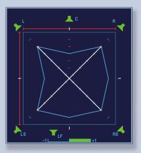
Same as the display on the left but with the phase of the left channel rotated through 180°. In the channel pairs L - R and L - LS each the correlation is r=-1 (hard inward broken TVI lines, red PSI lines and maximum spread of the PSI lines), a phantom sound source is not locatable.
